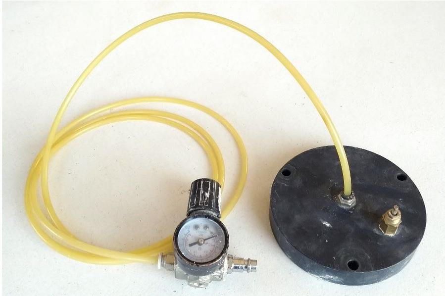
This is the endplate where the air comes in. A push connector holds the air line coming from the pressure regulator. I print at between 4 – 6 bar of pressure. The brass fitting to the right on the end cap is a safety pressure valve that that I am told will release pressure above 8 bar of pressure. A very important safety feature.
