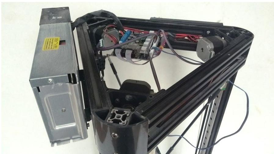
Follow the build instructions until you get to the Filament holder and Extruder motor. The filament holder is not attached and the Extruder motor, minus the mount is used to make the Clay Printhead - see next section. The Anycubic Plastic printhead is removed from the printhead mount plate and your Clay Printhead will later get attached to this plate. The plastic printhead is not used and is pre-assembled on the printhead plate that is attached to the diagonal rods.
