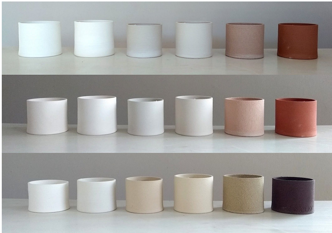
The six clay sample cylinder prints from left to right - China Clay, Porcelaine, Ball Clay, Smooth Stoneware,
