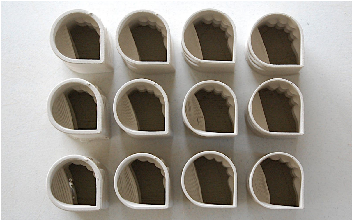
Nozzle size - (left to right) 3 mm, 2 mm, 1.6 mm and 1 mm.
