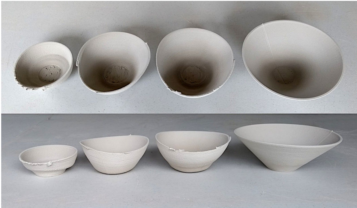
Clay Stiffness Test - hardest clay to the left softest to the right.
