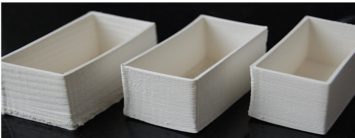
Soft/Medium print tests - over screwing on left hand print. Centre print, layer height 0.4, right print 0.35 mm
